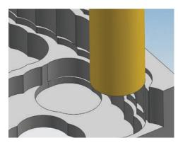
Specific plunge milling patterns apply efficient axial roughing to any geometry.
