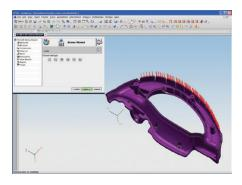
Designers launch the wizards from the Modeling application and work with the modeling part. When the chosen wizard is complete, the files remain loaded in the NX session so that the user can extend or review the work using either the Design Simulation or Advanced Simulation applications.
